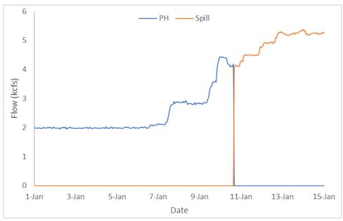
Figure 55. Hourly Flows PWR vs. Spill (Dexter Dam).
