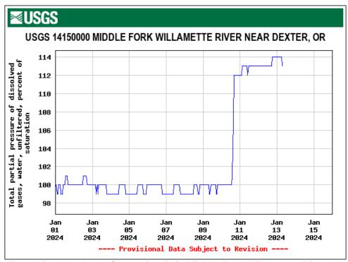
Figure 53. Total Dissolved Gas Saturation (%); Middle Fork Willamette River, Near Dexter, OR.
