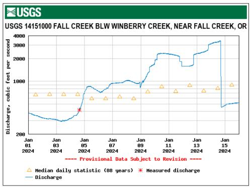
Figure 46. Discharge (cfs); Fall Creek Below Winberry Creek, Near Fall Creek, OR
