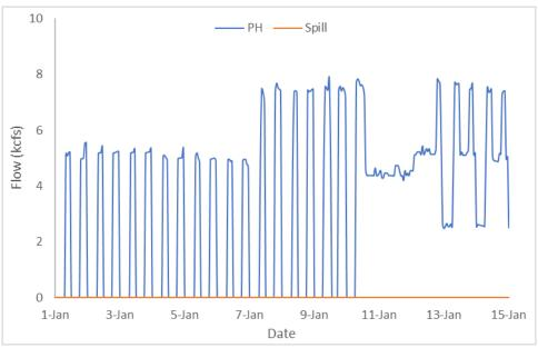
Figure 61. Hourly Flows PWR vs. Spill (Lookout Dam Tailrace).
