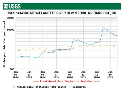
Figure 64. Discharge (cfs); above Lookout Point Reservoir, Below Oakridge, OR.
