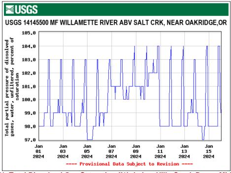
Figure 71. Total Dissolved Gas Saturation (%); below Hills Creek Dam – Middle Fork Willamette River.
